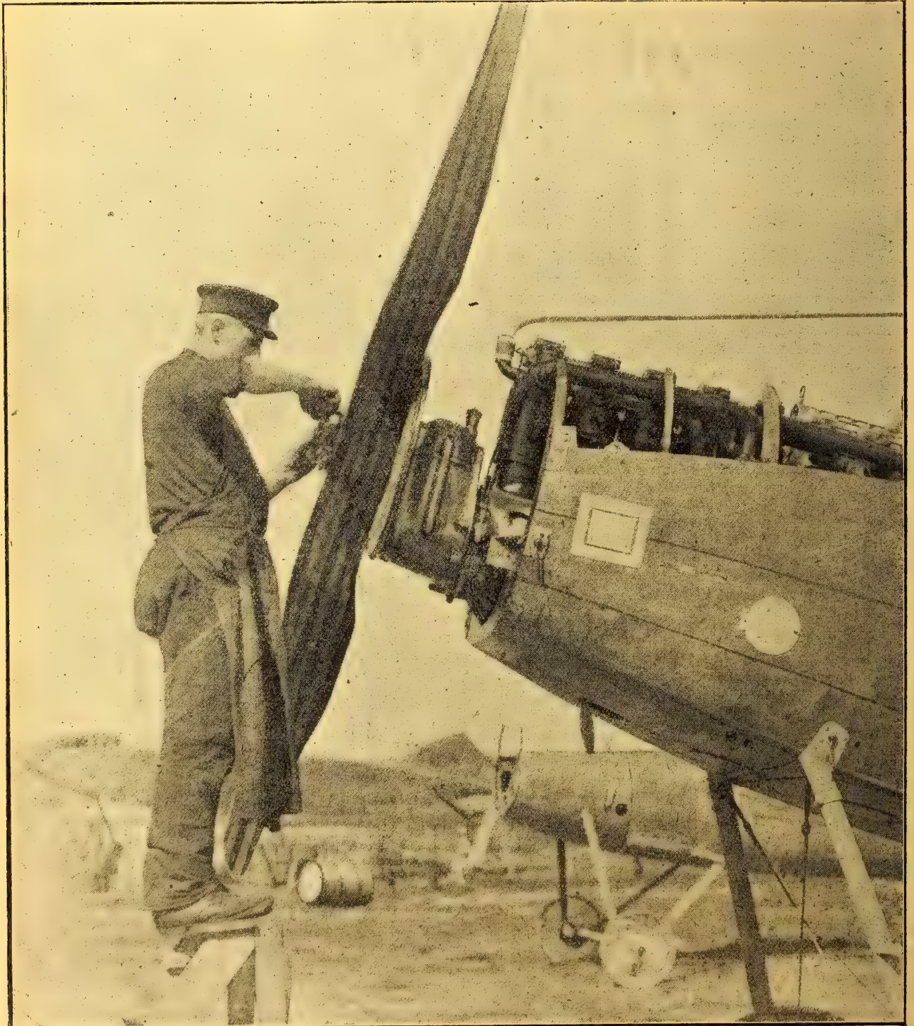
GERMAN AEROPLANES IN THE MAKING. —An interesting attempt to gear down an 8-cylinder Mercedes engine in an Albatros. The neat arrangement for the junction of the tapering wood fuselage, the cowl, the propeller, and the propeller pot should be noted, also that the centre of the propeller is cut away inside the cowling.
